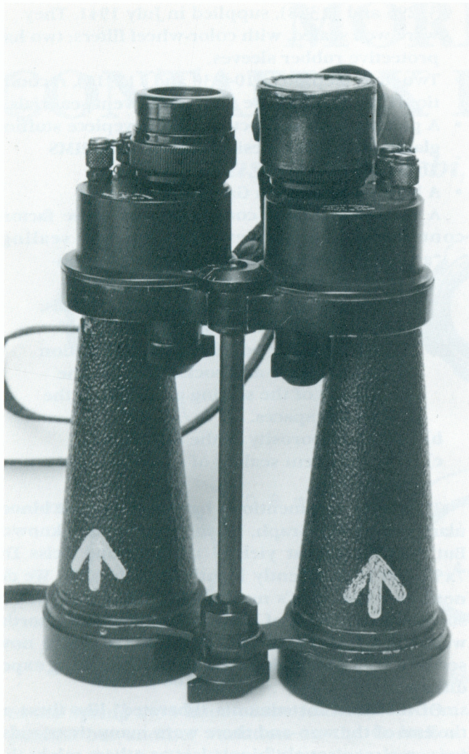
CF41 (#70119) manufactured in 1945 by Barr and Stroud, Glasgow and London. Designated as AP 1900A by the Admiralty, it was later renumbered AC 2021. Versions of the AP 1900 series remained the standard Royal Navy binocular until the 1979 introduction of the Avimo Binocular Prismatic General Purpose, 7x42 (Naval Service L11A1.) Desiccator vent-holes are sealed with screw-plugs secured by chains. In addition to indicating government ownership, broad yellow arrows show the tops of the barrels and make the instrument easier to see in poor light.
