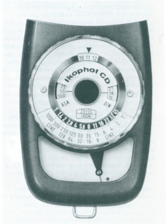
Ikophot S (left) was selenium; Ikophot CD used CdS Cell.
