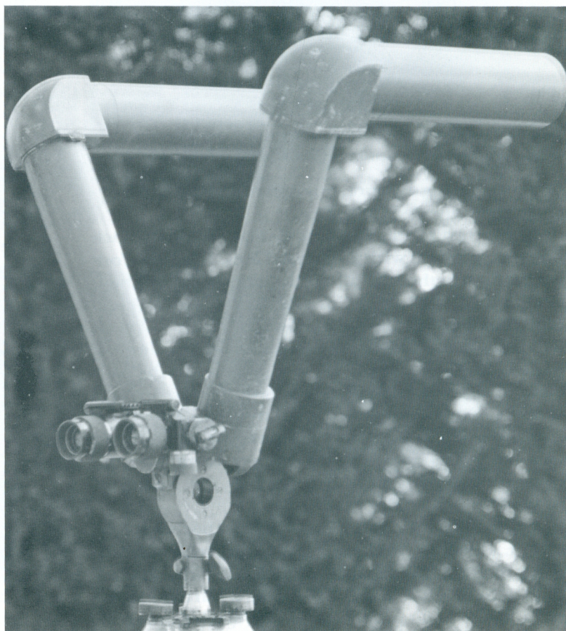
Unit opened into a "V". Long tubes protect the objectives from flare or rain.
