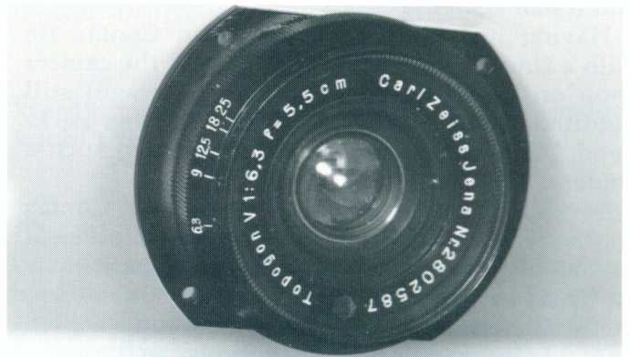
Topogon 5.5 cm f:6.3, probably for a Theodolite. Note European progression of f-stop markings, very unusual for a Zeiss lens of this era.
