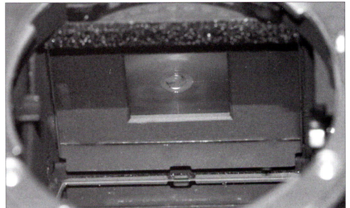
Above photo..A better view of the metal plate mounted below the focusing screen reducing its image to a square.
