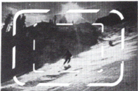
With Lens Field Selector set at "5", you see only the 50mm field of view. Setting the Selector to "8.5" adds the 85mm field, etc.
