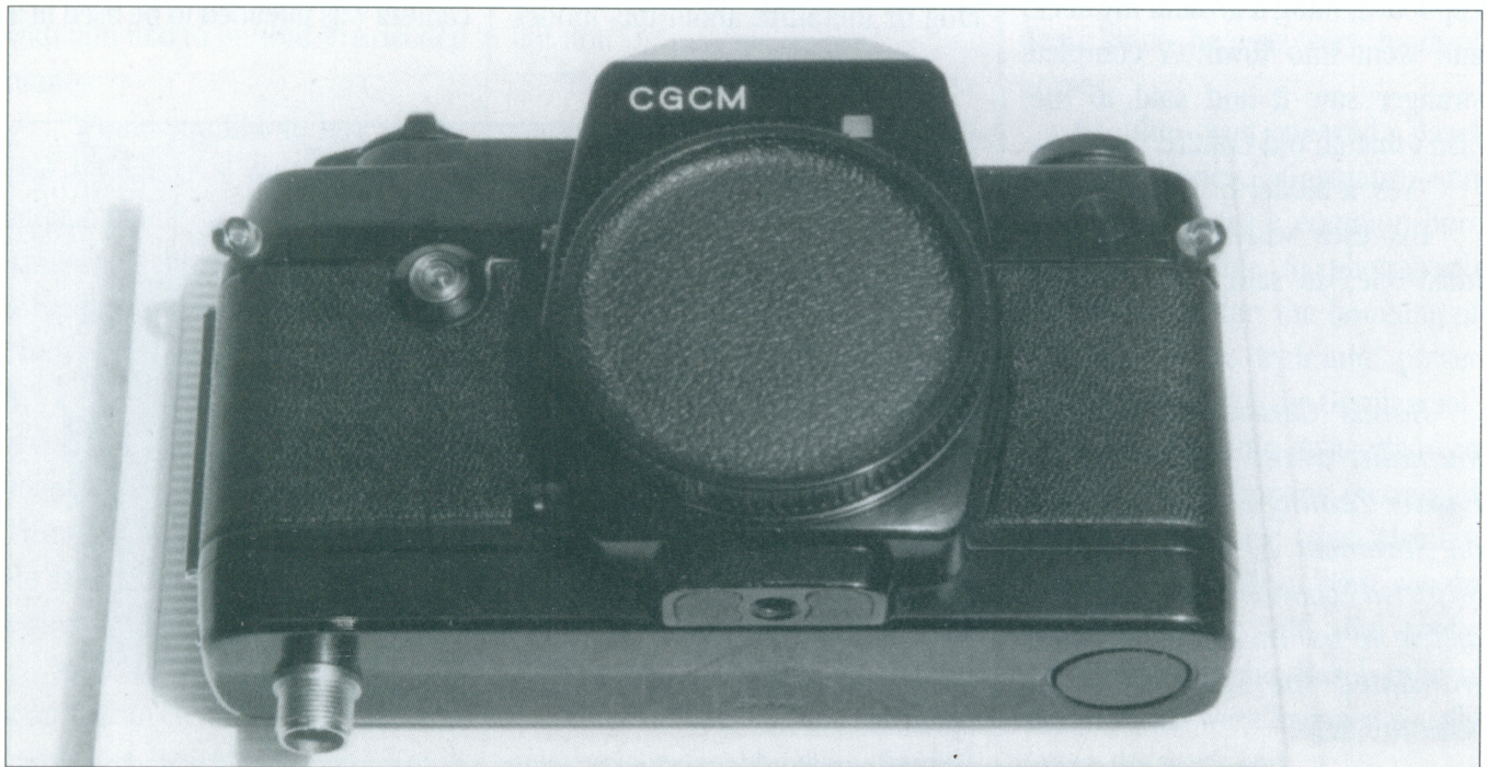
A modified Contax 137 MD shows a DIN type 5 prong plug built into the base of the camera.
