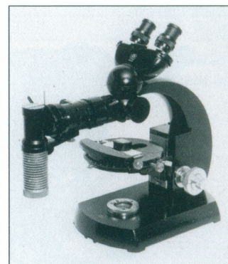
Carl Zeiss Standard Model WL with illuminator for reflected light. This special nosepiece is developed for studying opaque objects.
