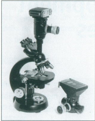
Carl Zeiss Model GF, a new trinocular tube for photomicrography, newly designed with interchangeable backs.
