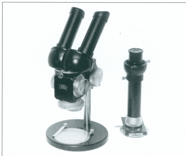
New Stereo microscope with interchangeable tubes. Monocular tube for photomacrography.
