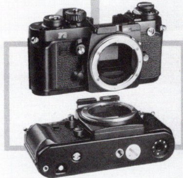
5. With the addition of the hot shoe, rewind knob, top covers and baseplate, plus grip and simulated leather covering, the F3 is near completion.
