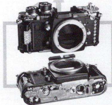
4. The mirror box, front body casting as well as the lens mount go on next.
