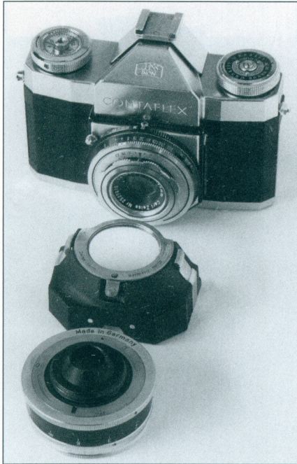
Easy to assemble, the auxiliary teleconverter and its mounting hardware form a rigid unit that transforms the Tessar into an 80mm portrait lens.
