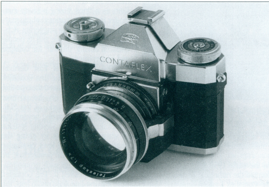
A Contaflex I with standard 45mm f2.8 Zeiss Tessar (top) and with the auxiliary Teleskop 1.7x converter (below) personify a Zeiss Ikon version of Clark Kent and Superman. The camera's outward and visible appearance changes dramatically when the Teleskop and its attaching bracket are put into place.
