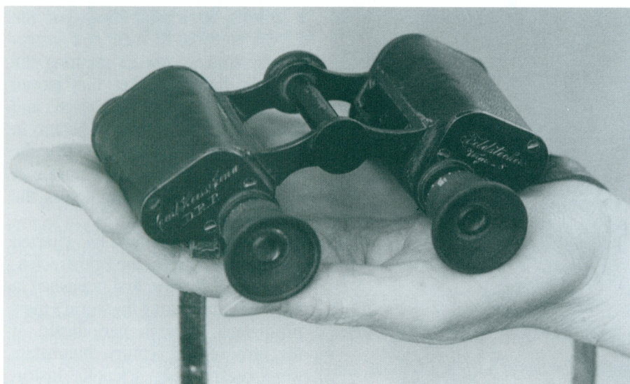
Figure 4. The diminutive Zeiss Feldstecher, the world's first successful prismatic binocular. It succeeded where Boulanger's instrument had failed, primarily because of its high optical and mechanical quality. This 8x20 instrument (Serial No. 1634) is an early example of the largest of the three models available.
