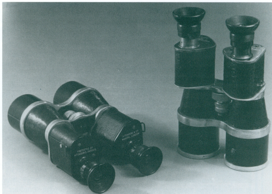
Figure 10. In Britain, Zeiss faced strong competition from several firms, including Aitchison, who introduced "large-diameter" (35 mm) objectives in 1903, four years before Zeiss. Though larger and more robust, their binoculars used the same basic layout as the Boulanger type (Figure 3). They were unique in having variable iris diaphragms. Here, 12x and 16x models are seen.
