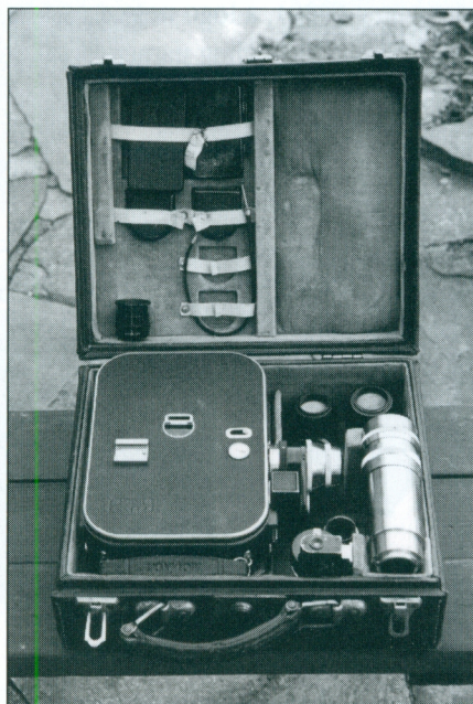
Outfit case as presented to me in 1980, with 18cm Tele-Tessar on right, filters and proxars in lid.
