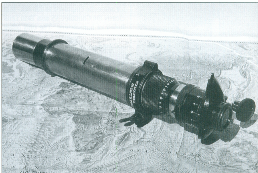
Another military item is this similar telescope which is estimated at being made between 1934 and 1945 for use in a naval application. It had both focusing and diopter controls.
